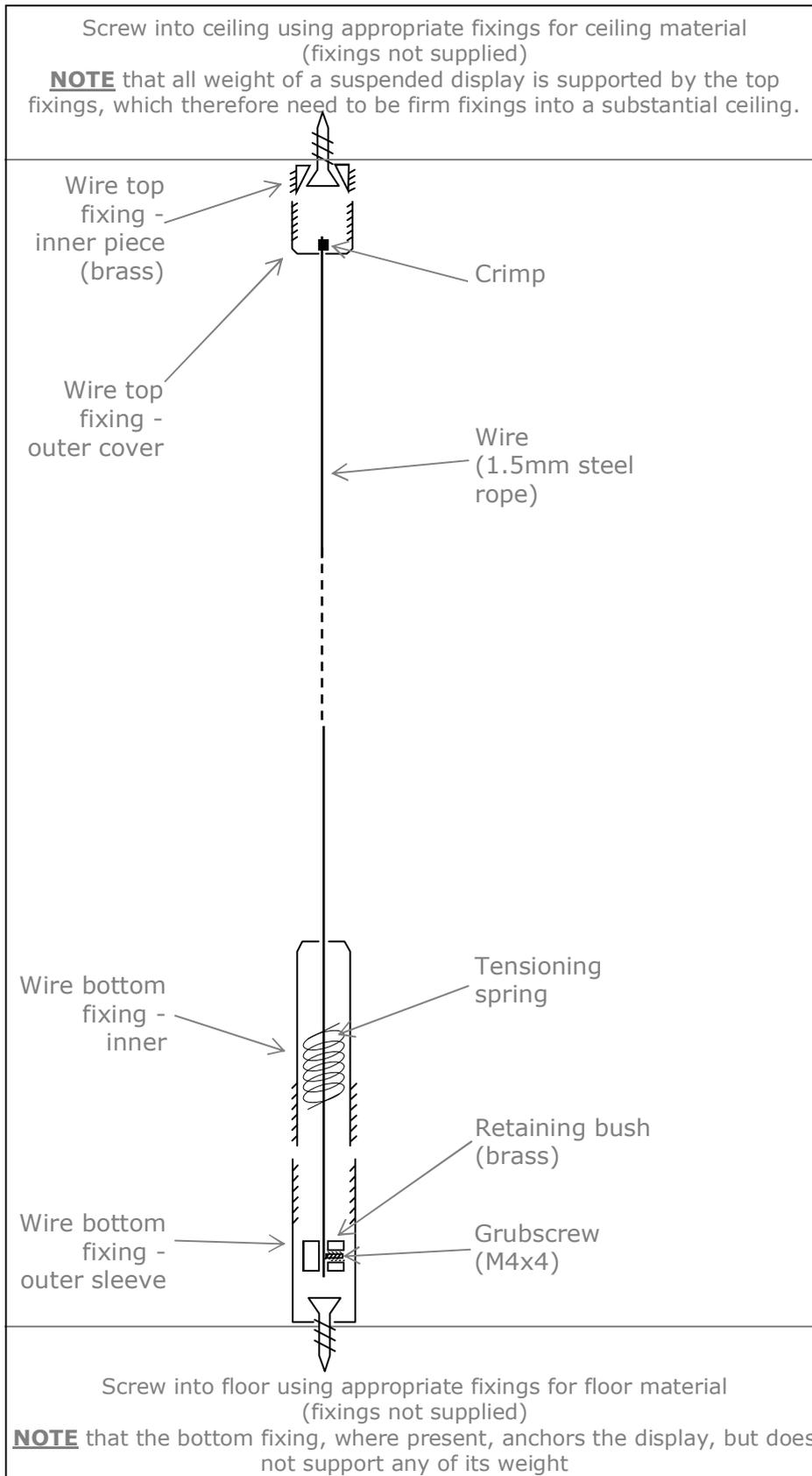
1. Mark the required positions of the wire top fixings on the ceiling. The table on page 3 shows the wire centres required for the different standard sizes of shelves.
