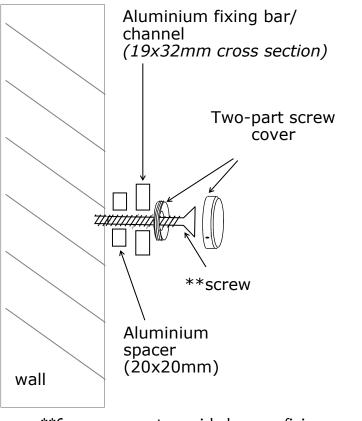
\*\*Screws are not provided - use a fixing appropriate to the surface to which the display is being fitted (board, brick, plasterboard etc)
