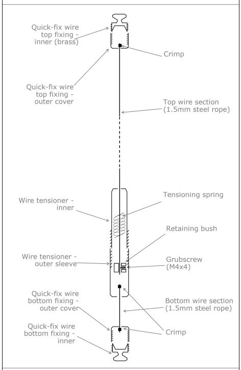
Quick-fix fixings slide into aluminium channel and can be secured in place by positioning appropriately then tightening up (by hand)
