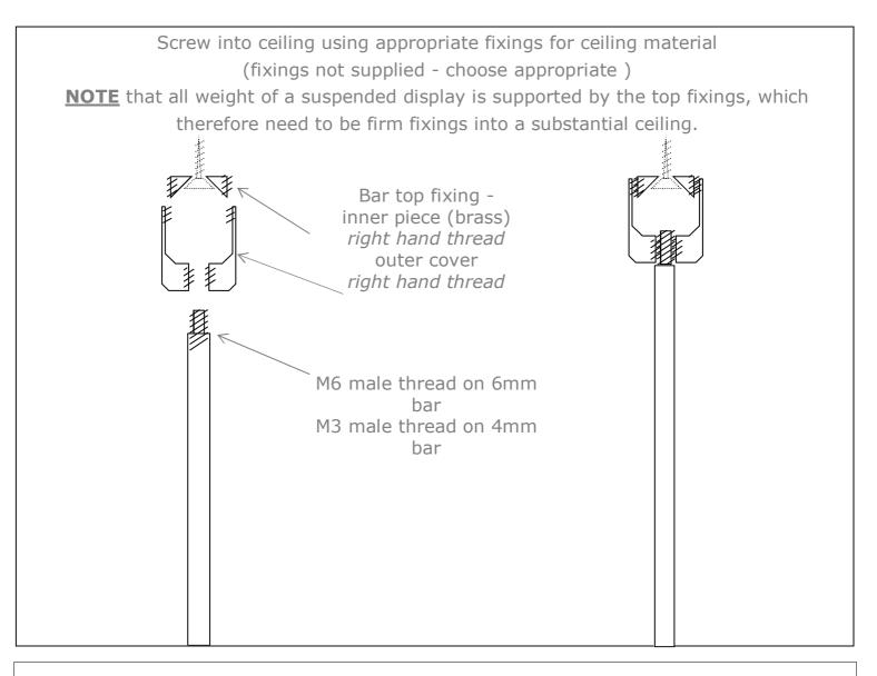
1. Mark the required positions of the bar top fixings on the ceiling. The table on page 2 shows the bar centres required for the different standard sizes of poster holders for both 4mm and 6mm diameter stainless steel bars.
