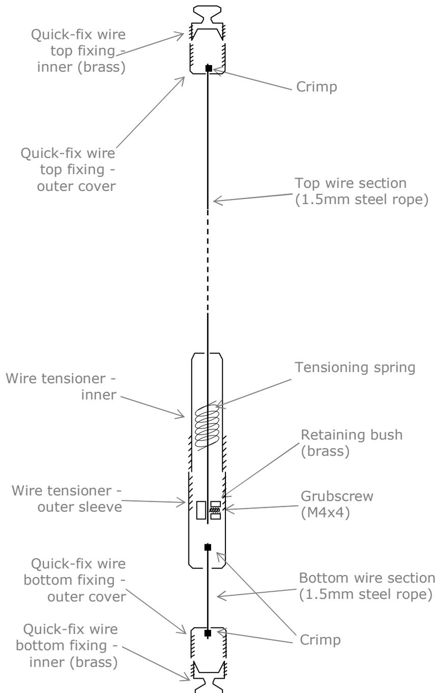
Quick-fit fixings slide into aluminium channel and can be secured in place by positioning appropriately then tightening up (by hand)
