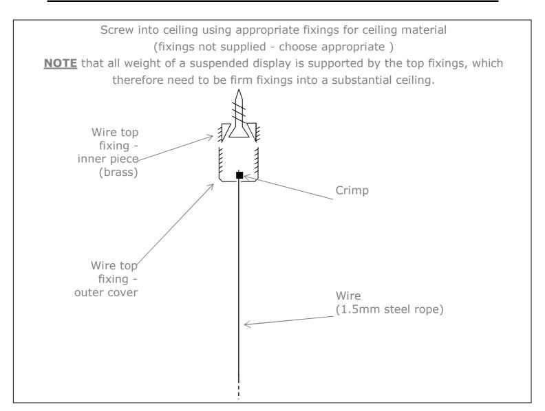
1. Mark the required positions of the wire top fixings on the ceiling. The table on page 2 shows the wire centres required for the different standard sizes of poster holders.
